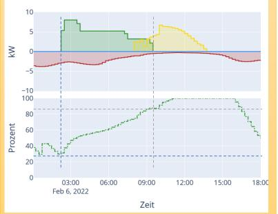
Simple two-point control leads to overheating of the storage tank (and to wasting solar energy)
